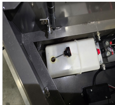
Reservoir fill location
