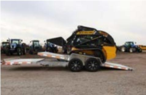
In a controlled manner, drive the equipment up on the deck. For single vehicles, the  $\frac{1}{4}$  turn valve can be left in the open position. As the vehicle moves up the deck, it will begin to lower automatically. If the  $\frac{1}{4}$  turn valve is in the closed position, the deck will not lower. This allows multiple smaller pieces of equipment to be loaded before lowering the deck.
