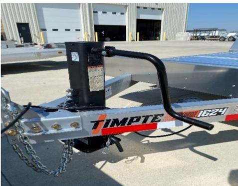
Raise the jack leg by turning the jack handle. Once the trailer is supported by the tow vehicle, pull the lower jack pin to raise the jack plate all the way up. Keep fingers clear of the jack plate.
