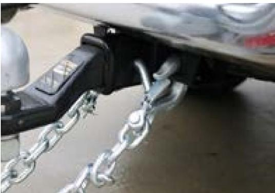
Next, attach the trailer safety chains to tow vehicle. Cross chains underneath hitch and coupler with enough slack to permit turning and to hold tongue up if the trailer comes loose.
