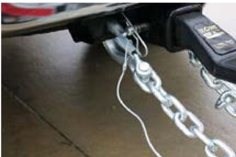
Attach the break-away safety cable to the tow vehicle.
